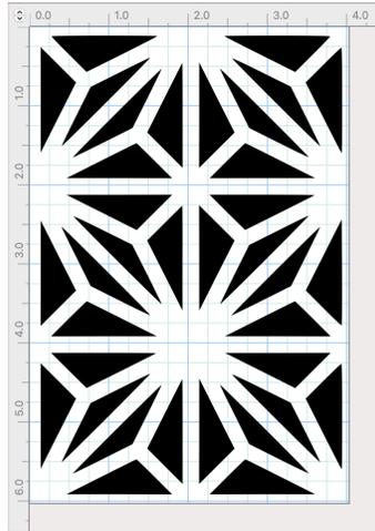
As with the small design, you'll notice is that the overall large design is not 4 inches by 6 inches (~100mm x ~150mm). Second, each of the triangles are 'bezier' curves, not straight sides. Each can be bent and curved after you click on it. Don't do that (for now). Select all the triangles and group them together; then 'lock' them.
