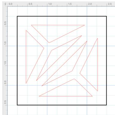
Export the stencil and square project to Glowforge. Place a piece of scrap proof grade material in the cutting area. Set the cutting sequence to do the triangles first (interior), then cut the square last.
