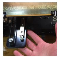
Turn the **Z-axis knob** to finish bringing the bed up until it almost touches the nozzle. (You should still be able to see a small gap at eye level, about the thickness of the sheet of paper.)
