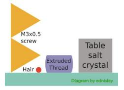
The **Z-EndStop** is set once before you begin printing, to lock the **Z-Home** value, so that the gap between the nozzle and the surface of the plate comes out to just at or below one layer height
