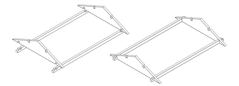
7. Glue the base top beams in place as shown below.
