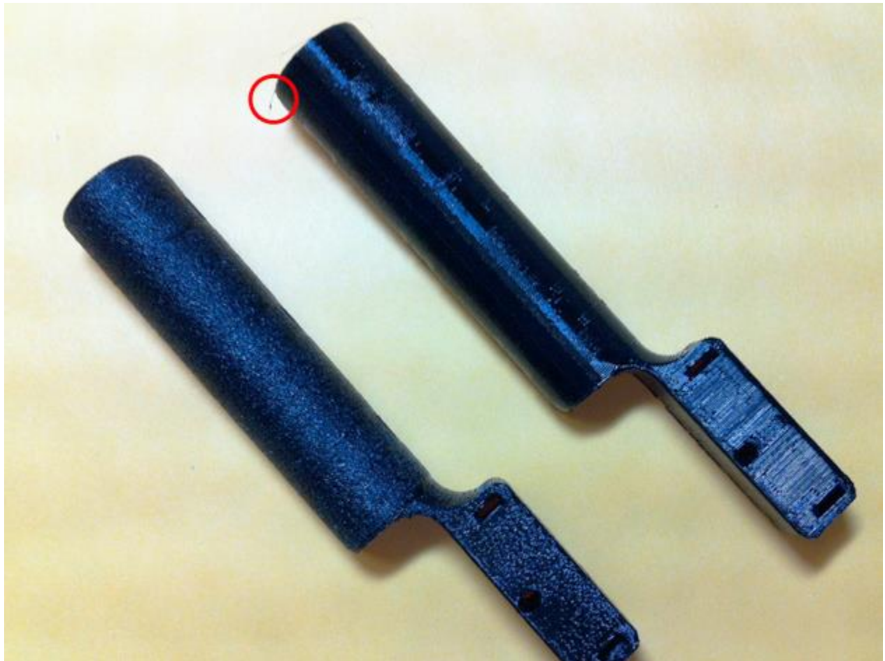
Normal extrusion on left, Slightly under-extruded on the right. Both prints are fully functional, but the left version is literally covered with thousands of tiny threads that wrapped around the print making the surface rough and glittery. The one string on the under-extruded print is the one that was left at the very end, when the bed moved down. PETG_underextrusion_comparison.jpg (277.11 KiB) Viewed 42765 times
