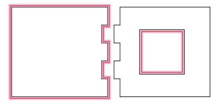
Cases where you might want to consider adjusting for the kerf would be inlay work, parts that need to end up being very specific sizes, miniature work, and anything designed by an engineer. (Occupational hazard.)
