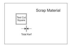
(Note: The kerf changes at the top and the bottom of the material, depending on where the laser is focused in the material. The most accurate place to focus the laser for kerf measurements is at the midpoint of the material. Then the kerf at the top and the bottom are closest to being equal.)
