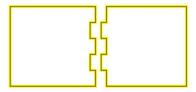
If we designed our parts to be exactly 100 millimeters wide, and they <u>have</u> to be that width in order to fit together properly, we will have to shift the design lines out further by <u>half the width of the kerf</u> in order for the end result to wind up at exactly 100 mm. That will cause the edge of the laser beam to just kiss along the originally designed line, instead of the center of the beam. Then the actual part will come out to be the correct size.
